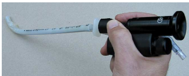
Fig. 1 The FPS scope with the miniature LED light source held in a pencil grip manner. The LED is turned on and off by rotation of the round knob below the eyepiece. Full counterclockwise rotation unscrews the cap entirely to change the N-sized battery.
