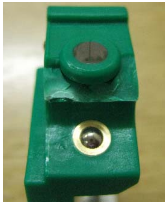
Photographs showing failure site on blade retention mechanism on Sample 10
