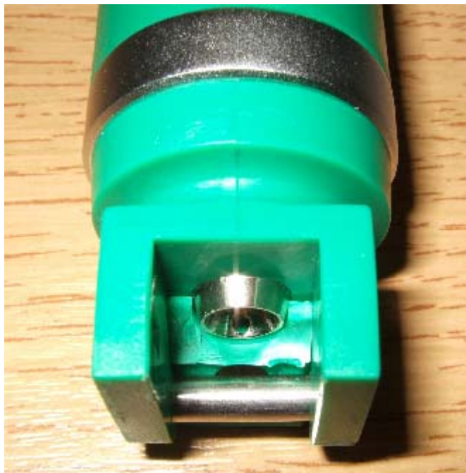
Photographs showing failure site on blade retention mechanism on Sample 10
